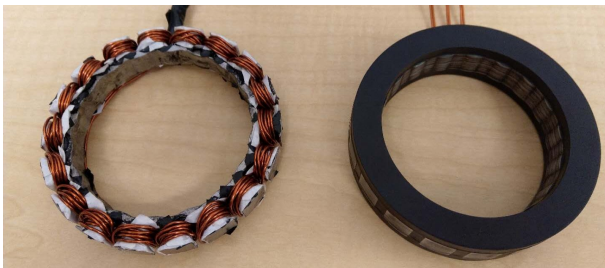
Fig. 5. A comparison between a stator with (right) and without (left) encapsulation technology. Left: a stator without encapsulation, where the white part is the isolation layer made of nylon material. Right: the designed stator with encapsulation, which is the black material.
