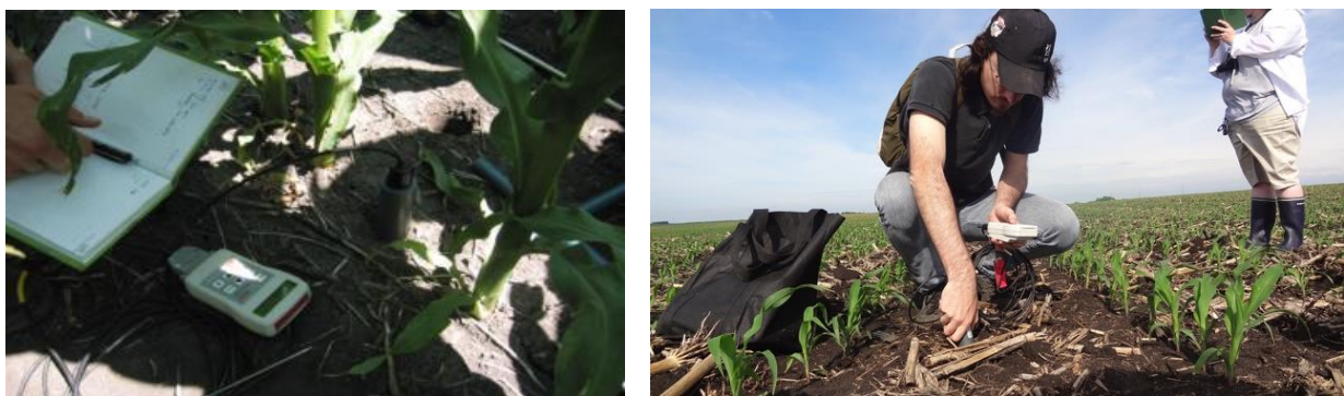
Figure 24: Coincident to gravimetric methods, impedance probe measurements help to improve efficiency of sampling on the ground.
