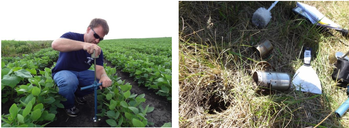
Figure 23: Gravimetric sampling, where a surface soil core of known volume is collected at multiple depths for comparison to aircraft and satellite products.
