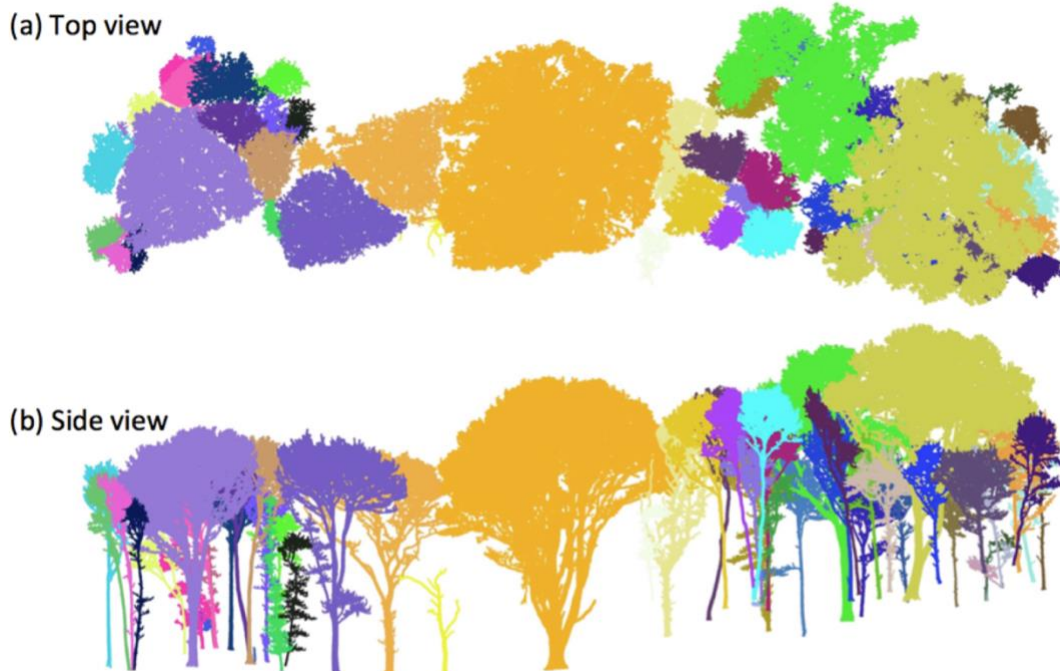
Figure 2.4 Example of a co-registered and segmented TLS point cloud from Wytham Woods, UK. Single trees extracted for a 20 x 100 m transect. Data captured with a RIEGL VZ-400 instrument and tree extraction was done with the treeseq algorithm (Burt et al., 2019). (a) Top view; (b) Side view
