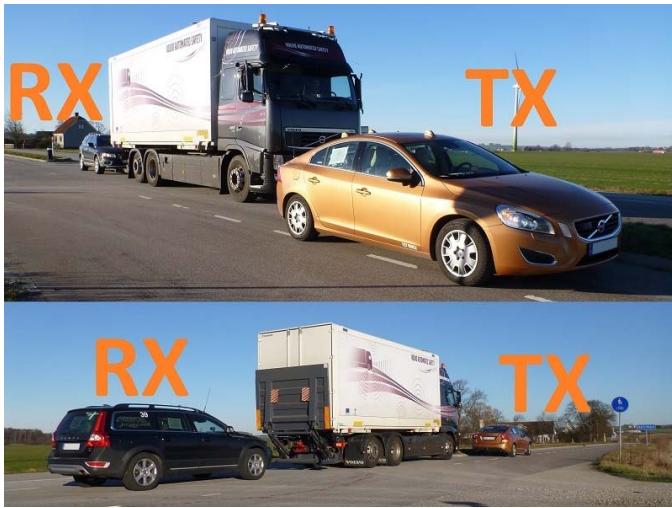
Fig. 1: The two cars at TX/RX and the truck as obstacle used in the measurements. The total truck length was 980 cm with a container width of 260 cm and height of 400 cm from the ground.
