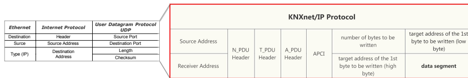
Figure 5: KNX packet encapsulated into a TCP/IP packet.
