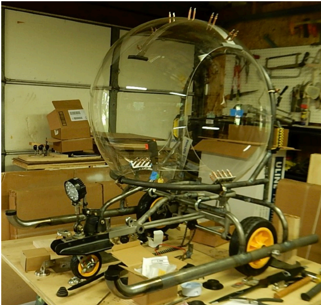
Clecos were used to clamp the aluminum re-enforcements prior to riveting.
