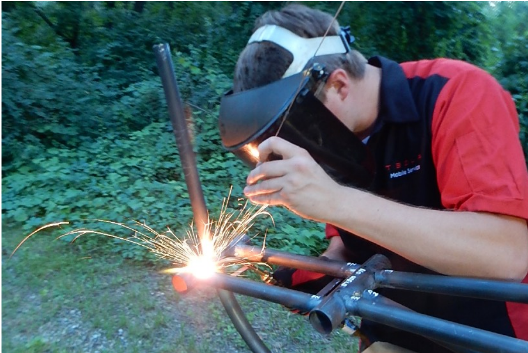
Tony is finishing a weld at the terminator tube on the tail post.
