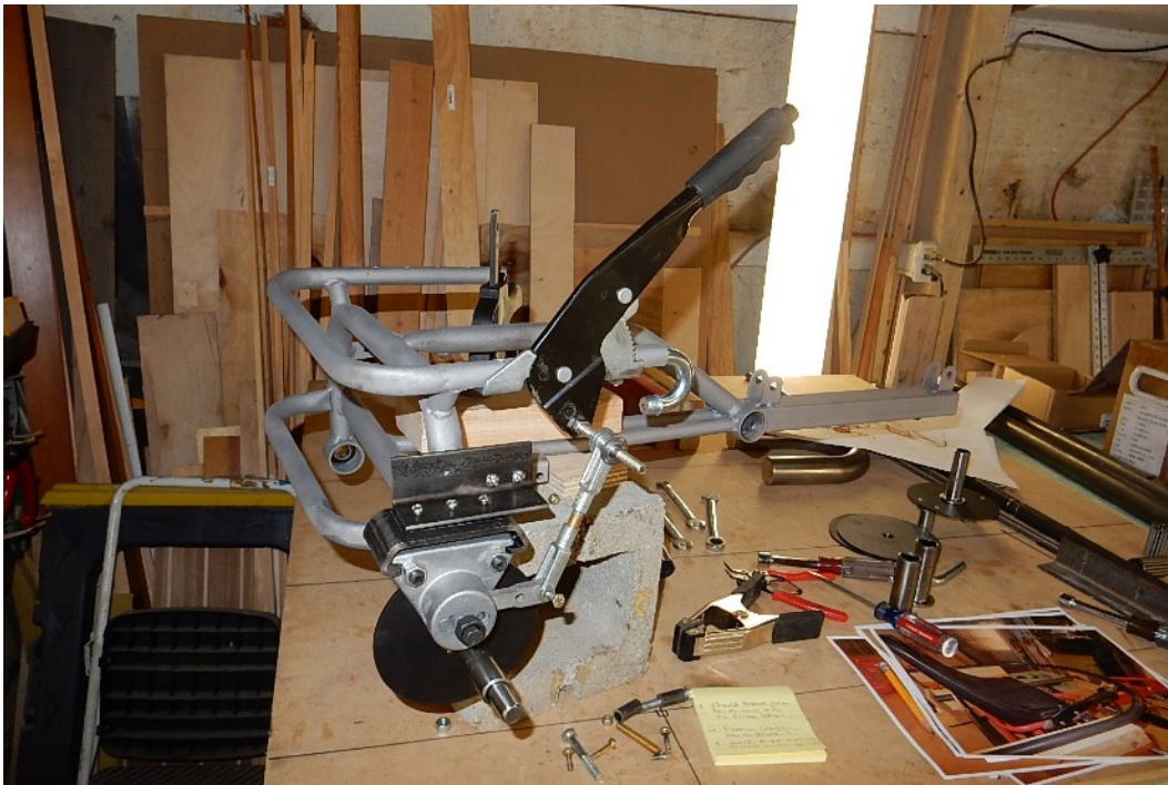
A Go-Cart disk brake is connected to the cart frame along with a ratcheting short brake lever.
