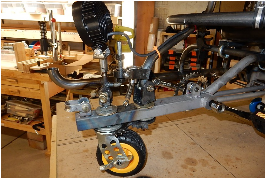
A spring was added to give the stick pull back pressure.
