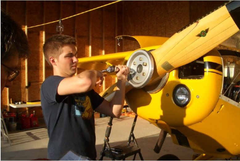
Photo B -Tony torquing bolts on the prop hub of my PA-14.
