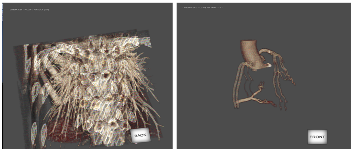
Figure 13. Unclear left- and right-view separation resulting from failed eye tracking. The resulting 3D crosstalk manifests as overlapping double images and 3D fatigue for the user.
