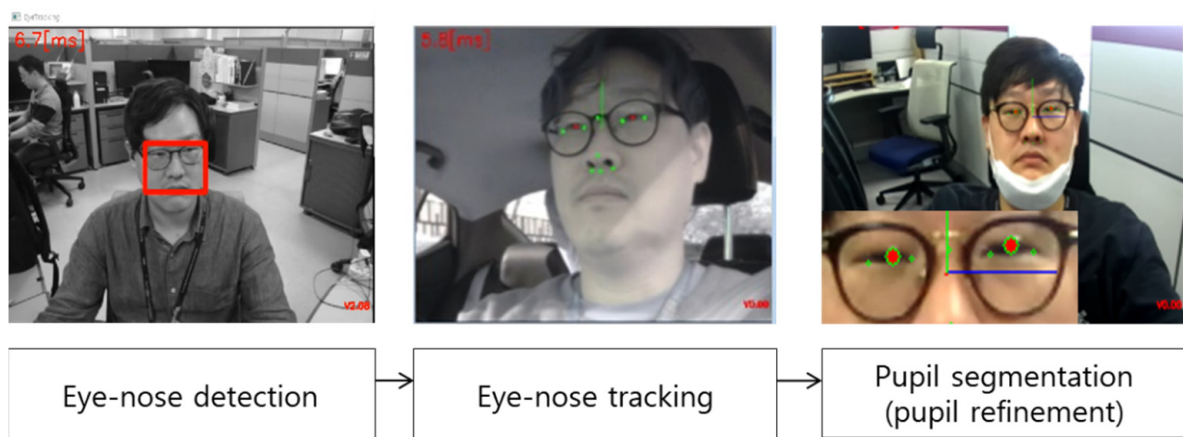
Figure 5. Illustration of the proposed eye tracking method, which includes pupil segmentation modules. The left image shows an extracted subregion (red box) including the eyes and nose of the subject. The middle image shows the 11 landmark points (green dots) used to inform the Supervised Descent Method (SDM)-based shape alignments. In the right image, the green circles around the red points on the eyes indicate the pupil segmentation modules, which increase the accuracy of the eye tracking.
