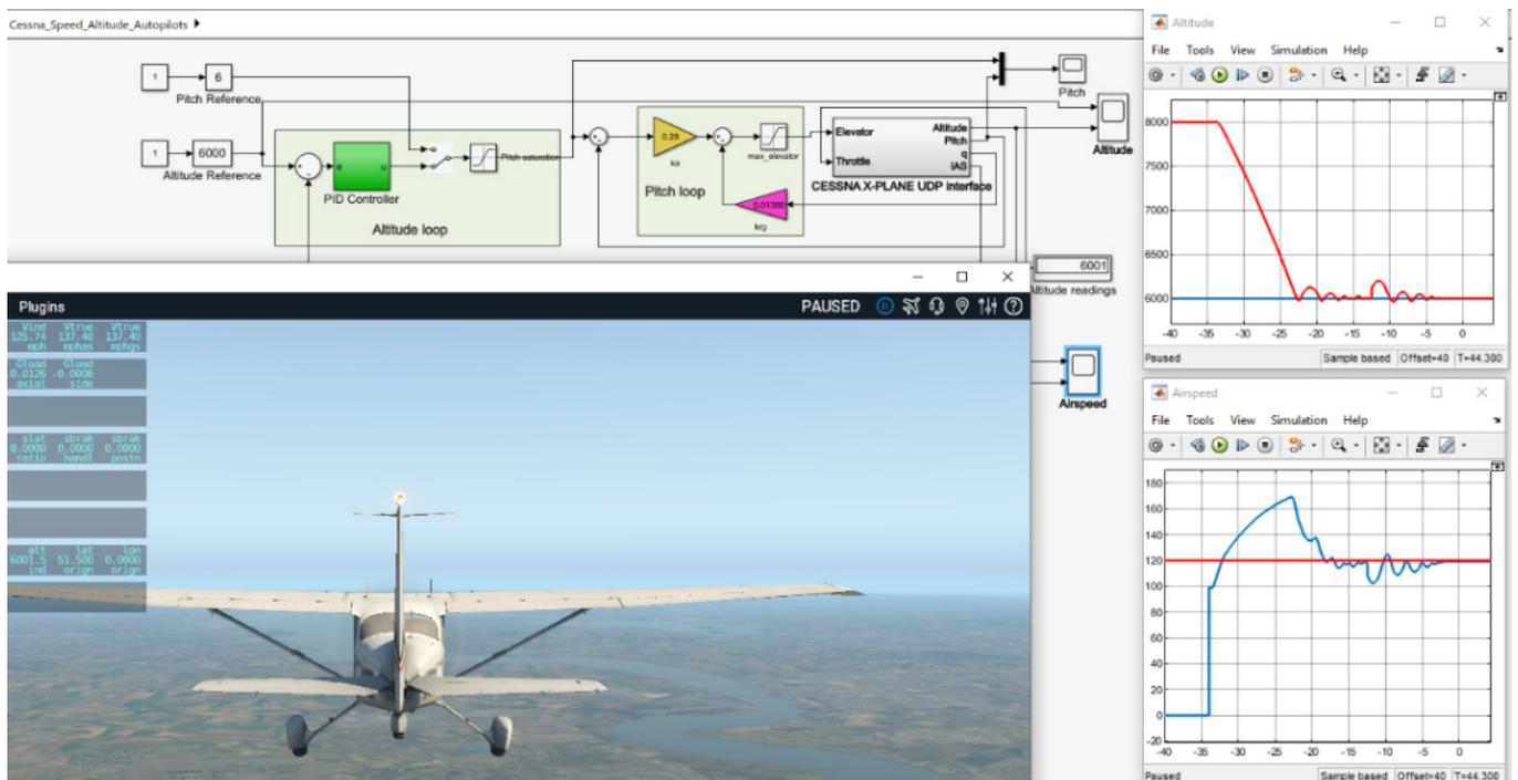
**Figure 8.** Flight co-simulation using Matlab/Simulink and Xplane.
