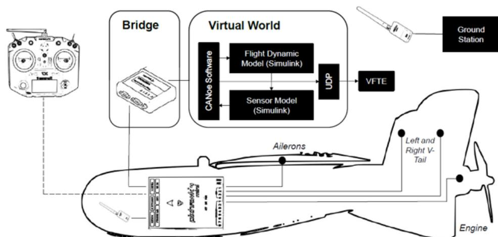
**Figure 23.** HIL architecture using Pixhawk (courtesy of Alphalink Technologies Inc.).
