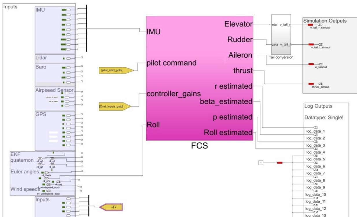
**Figure 20.** Example Nano Talon flight control model for Simulink/VFTE lateral flight co-simulation (Developed from Alphaslink Technologies Inc. (Newark, OH, USA) training resources).
