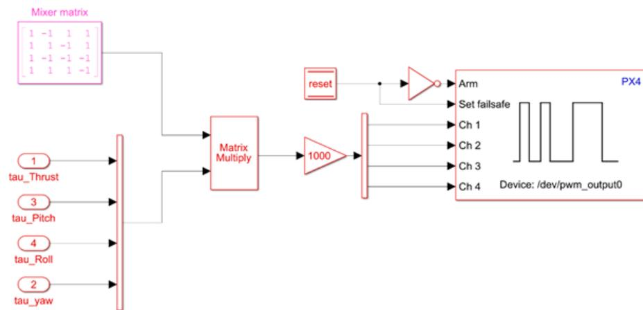
**Figure 18.** Control channels allocation/mixing for the X-configured quadcopter SIL position tracking example by The Mathworks, Inc. [28].
