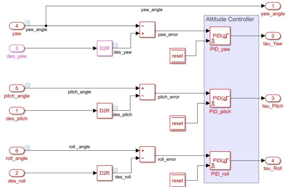
**Figure 17.** PID autopilots in the X-configured quadcopter SIL position tracking example by The Mathworks, Inc. [28].
