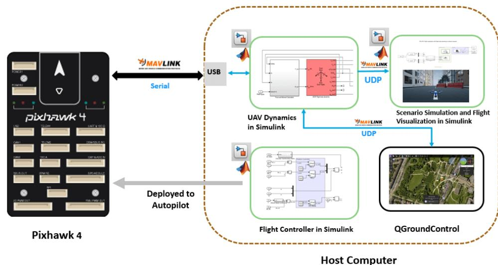
**Figure 19.** HIL simulation architecture using a Pixhawk 4 with a Simulink-Unreal Engine co-simulation [29].
