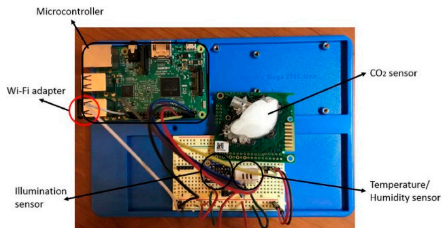
Figure 7. The integration of three sensors in Ref. [105].
