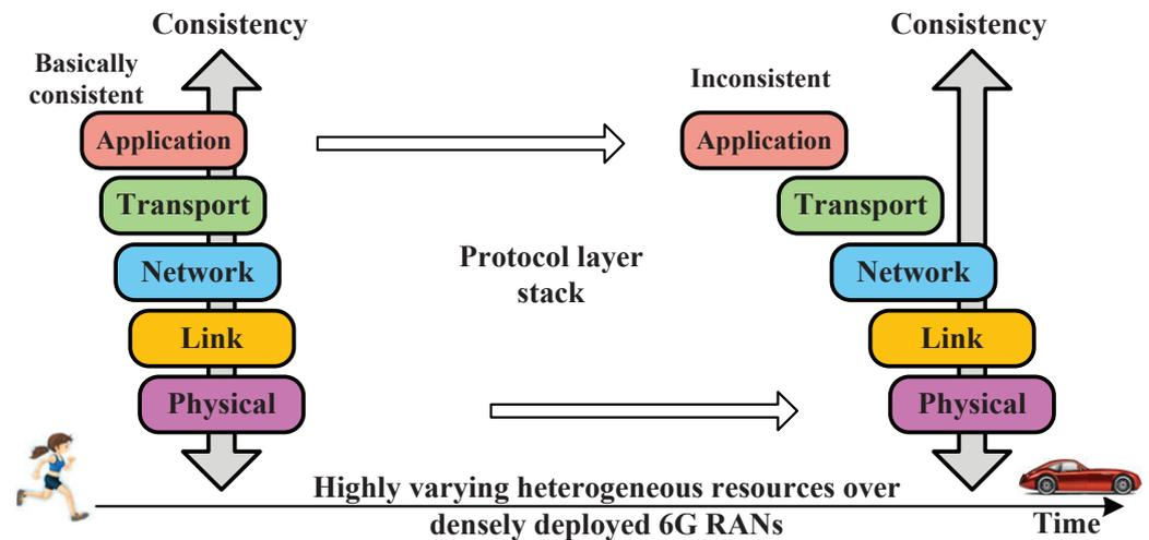
**Figure 5.** Inconsistent responses to the highly varying heterogeneous network status caused by the loosely coupled protocol stack.
