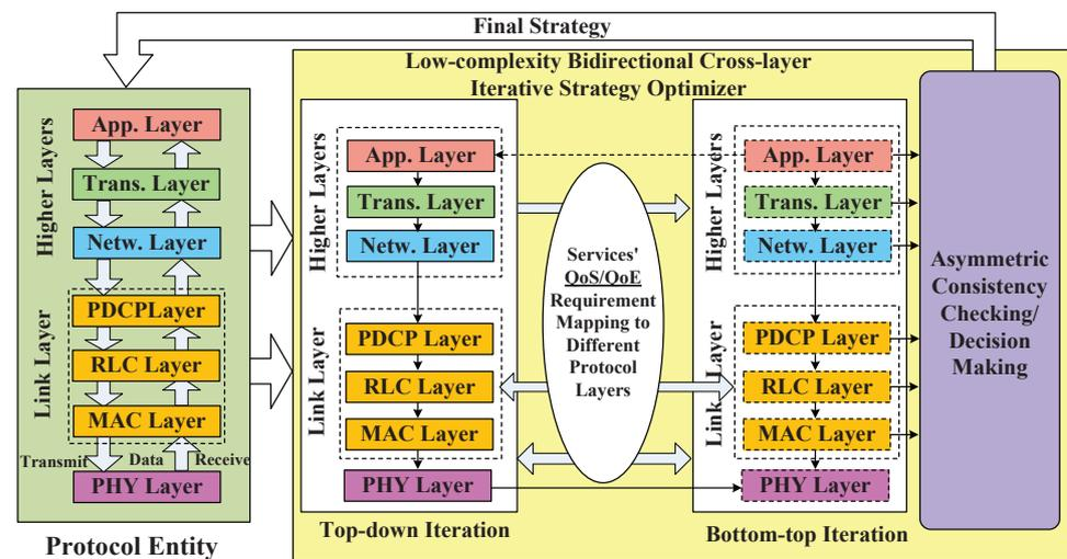
**Figure 6.** Tightly coupled cross-layer framework with service-awareness achieved via bidirectional iterative strategy optimization (using the typical architecture of a protocol stack in 3GPP as an example).
