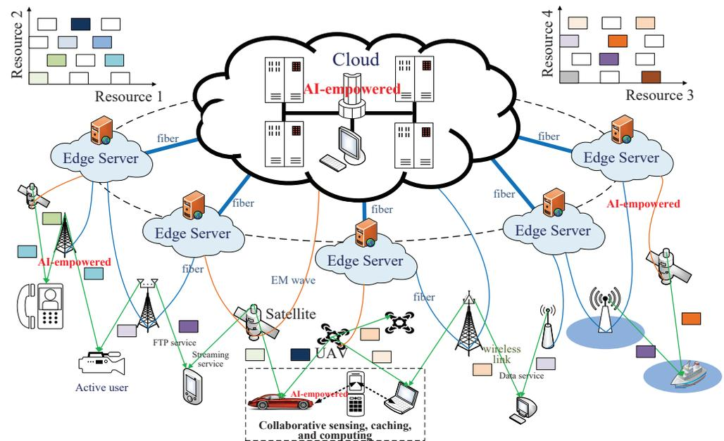
**Figure 3.** Intelligent cloud architecture for the 6G RAN.
