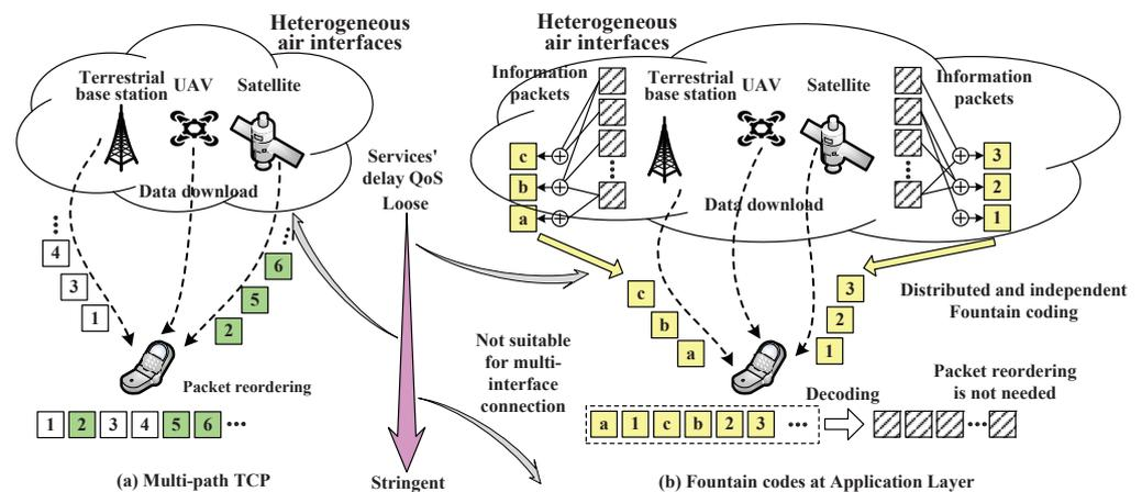
Figure 8. Service-aware access of heterogeneous RATs: the multi-path TCP approach and fountain-code-based approach.
