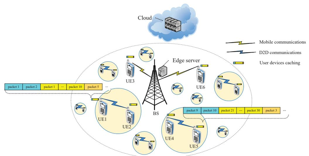
**Figure 9.** Atomized caching enabled by fountain codes with support by D2D communications and user socialization.
