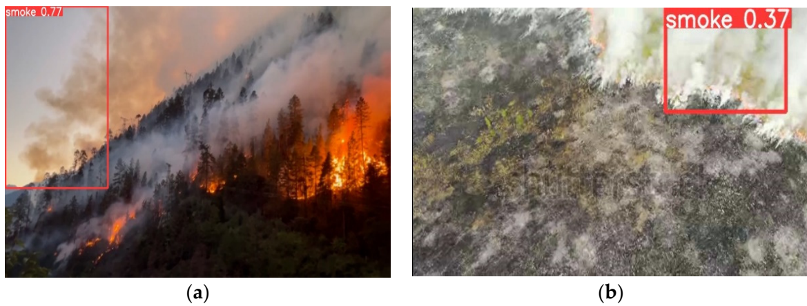
Figure 6. First-stage smoke detection and some experimental results: the model can detect specific colors of smoke (white smoke) due to the limitation of the dataset ((a) model 1 and (b) model 2).
