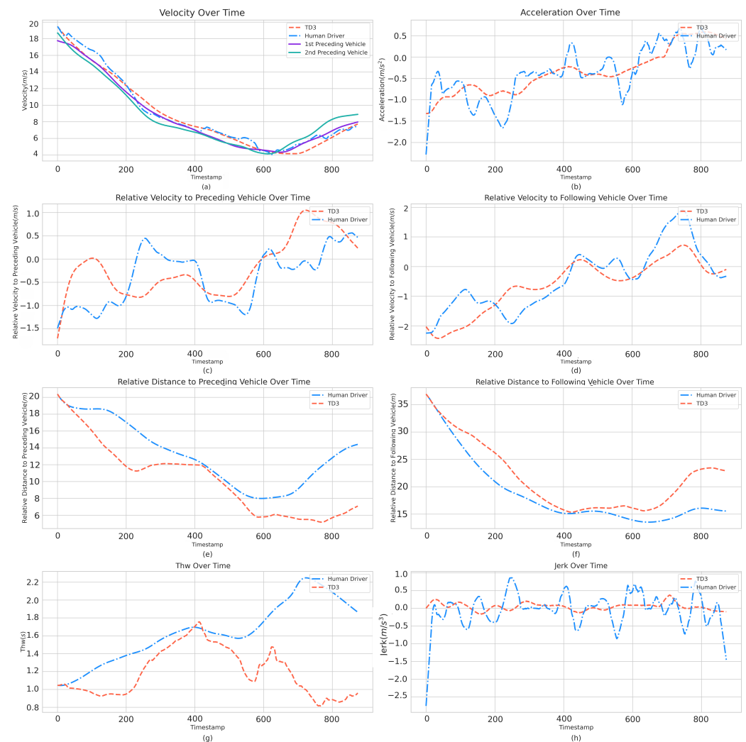
Figure 10. Comparison of performances between the TD3 agent and human driving on the scenario with SV no. 2742, 1st preceding vehicle no. 2738, 2nd preceding vehicle no. 2736, and 1st following vehicle no. 2744 of track 25 in the test dataset. (a) Velocity. (b) Acceleration. (c) Relative velocity to preceding vehicle. (d) Relative velocity to following vehicle. (e) Relative distance to preceding vehicle. (f) Relative distance to following vehicle. (g) Thw. (h) Jerk.
