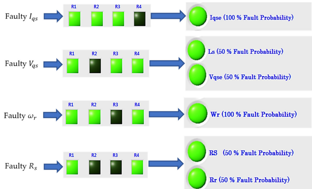
Figure 12. HMI for different residual conditions under fault.
