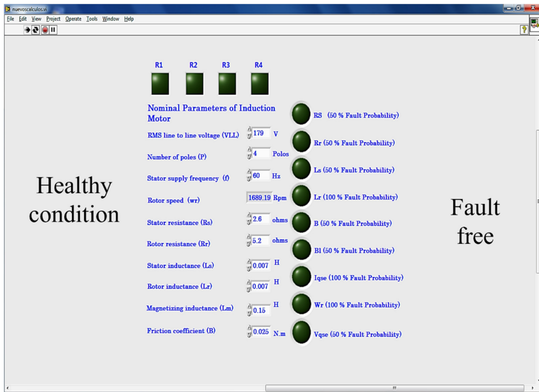
Figure 11. Screen of HMI for the 3PIM fault detection in the fault-free case.
