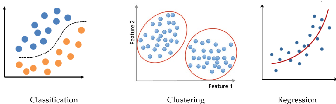
Figure 13. Basic machine-learning tasks: classification, clustering, and regression.
