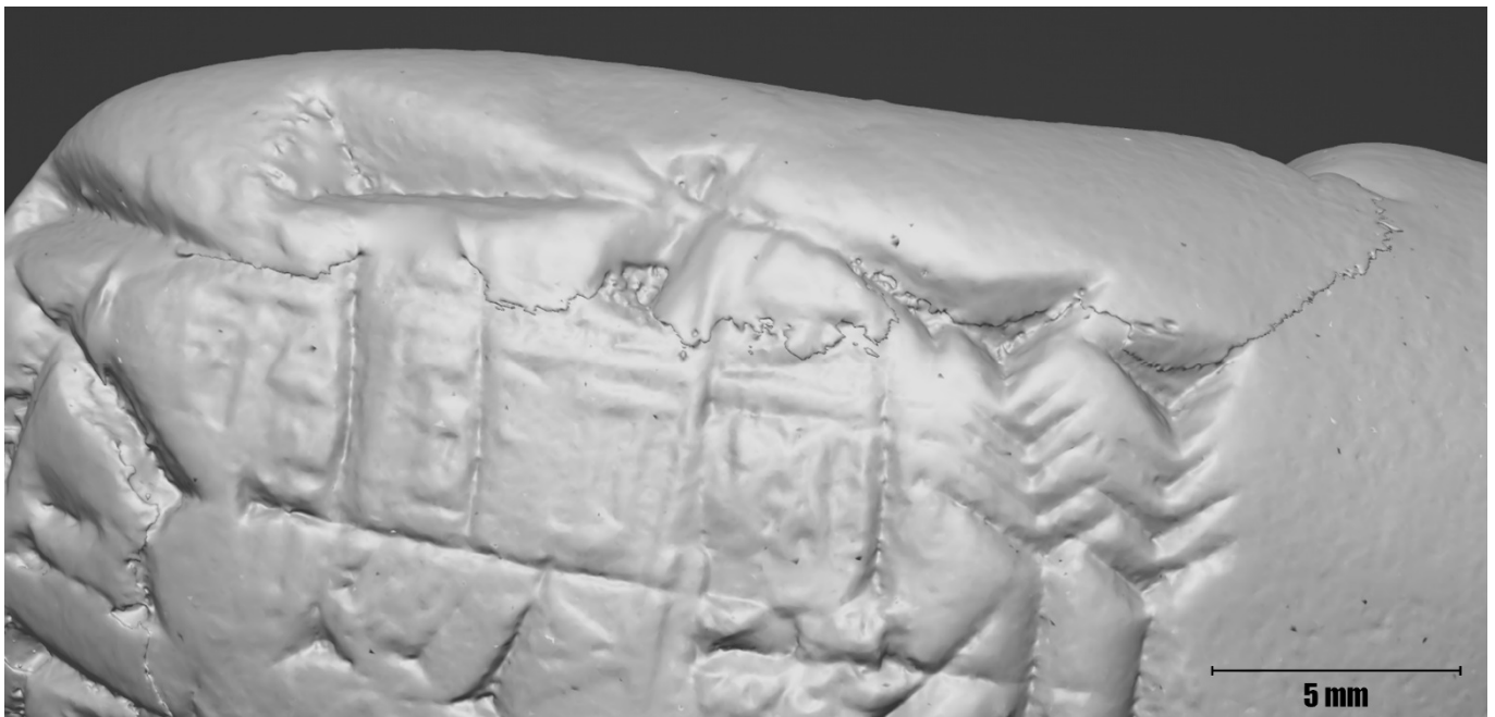
Figure 21. Detail of the mesh obtained by joining two partial models; evident is the stitching of the two pieces, which can be smoothed in post-processing.
