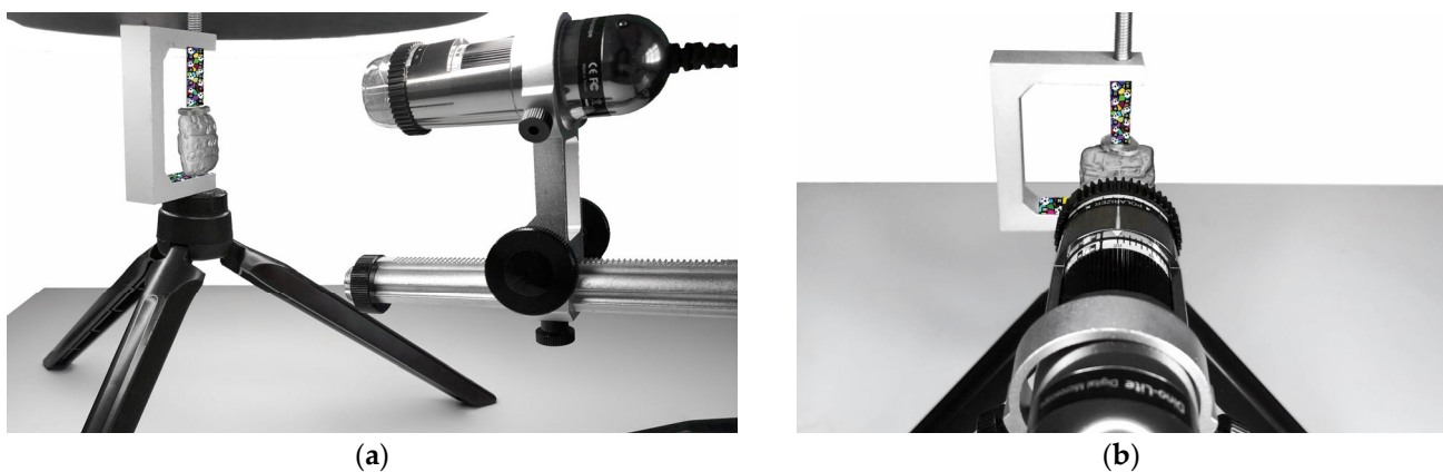
Figure 12. The second acquisition configuration with the screw clamp: (a) the screw clamp coaxial to the rotating base; (b) detail of the positioning of the tablet in the clamp.
