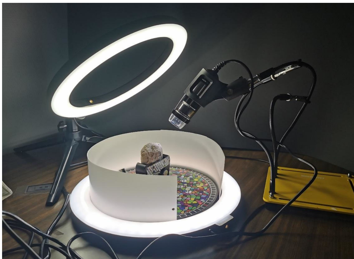
Figure 20. Acquisition system based on the turntable and clamp with ring illumination to support the microscope-integrated LED illumination. Magnification related to working distance: 20×.
