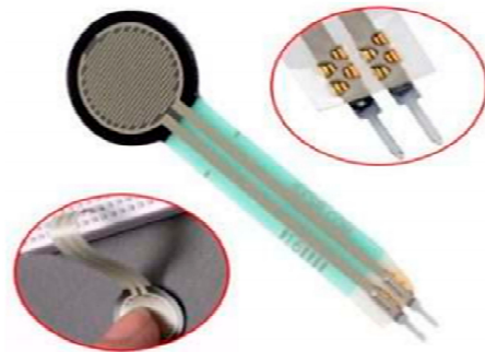
Figure 6. Tactile sensor or force resistive sensor [101].
