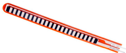
Figure 5. Flex sensor or bend sensor [12,14,26].
