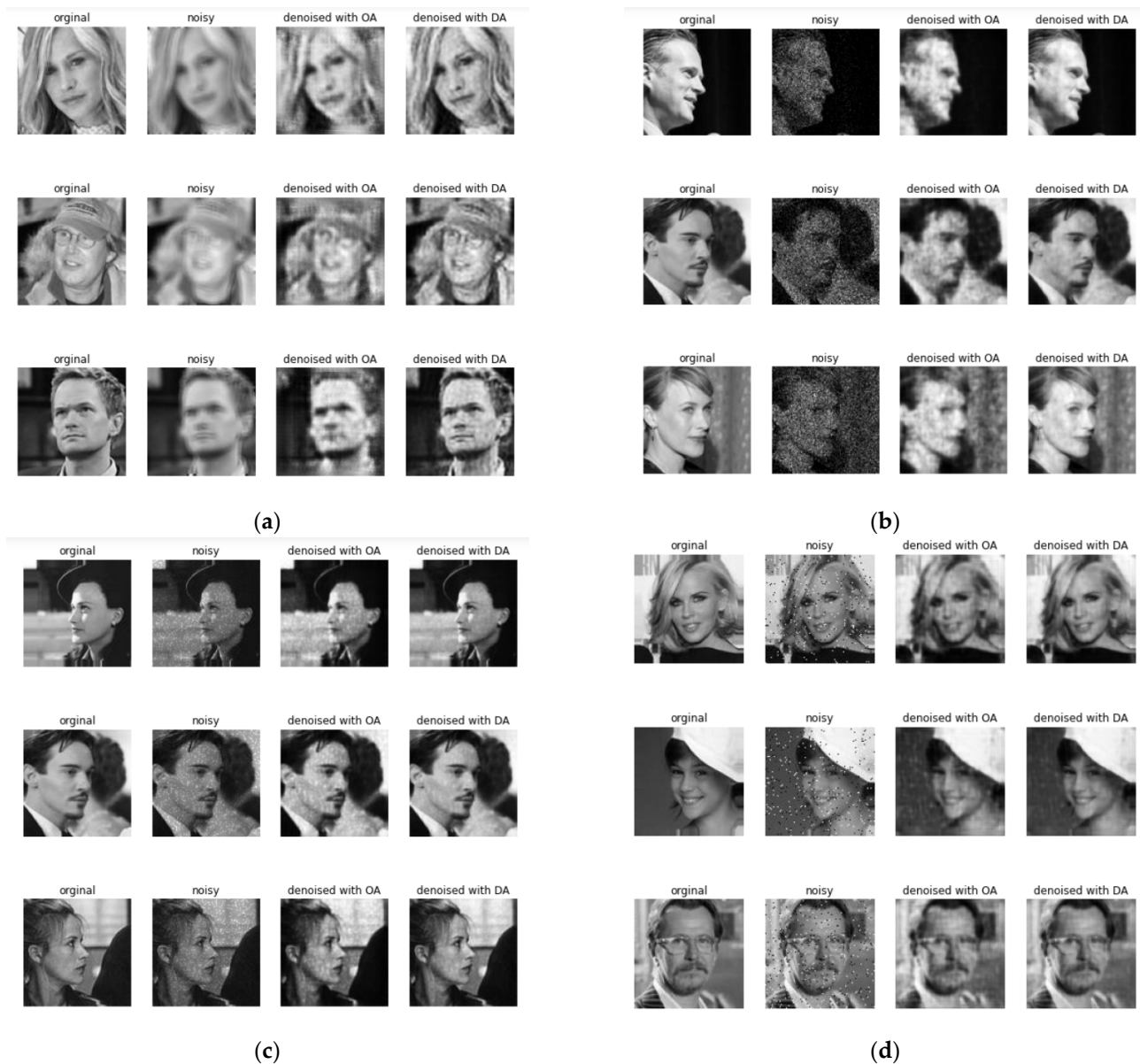
Figure 13. Original image [68–71], noisy image, and images restored by one and dual autoencoders with separable convolutional neural networks under (a) Gaussian noise, (b) Poisson noise, (c) speckle noise, and (d) impulse noise.
