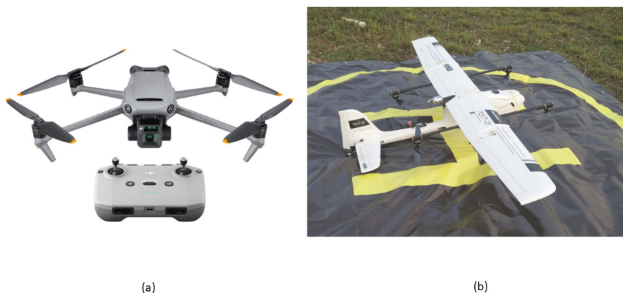
Figure 2. A high-quality image of (a) quadcopter/multi-rotor and (b) fixed-wing UAVs.
