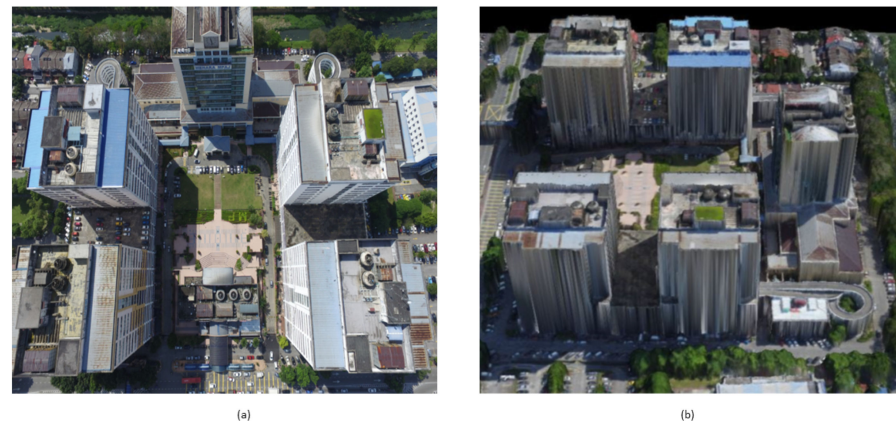
Figure 4. Type of imagery (a) 2D aerial imagery acquired via UAV; (b) 3D model built from UAV imagery.
