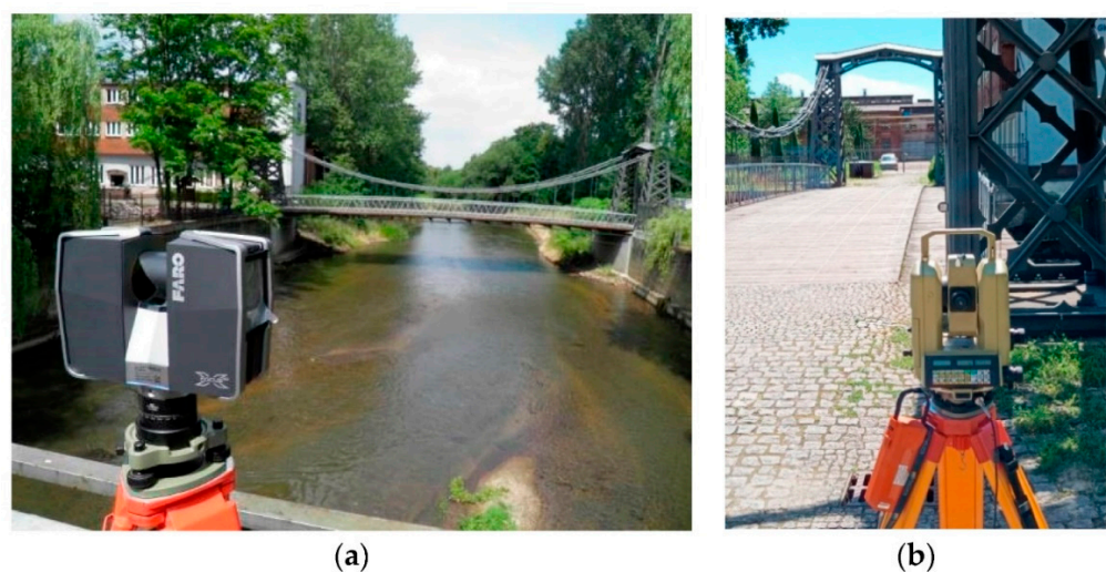
Figure 1. A typical TLS: (a) FARO Focus 130 3D laser scanner; (b) Leica TC2002 total station [20].
