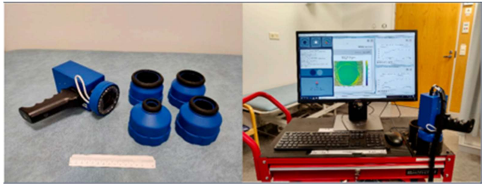
Figure 5. SICSURFIS handheld hyperspectral imaging system [40]. The article [66] describes the principle and testing of the first phase of a three-stage pilot of this imaging system, focused on the intricate skin surface. The device is still a prototype and ongoing refinement is needed before it can be used for clinical applications.
