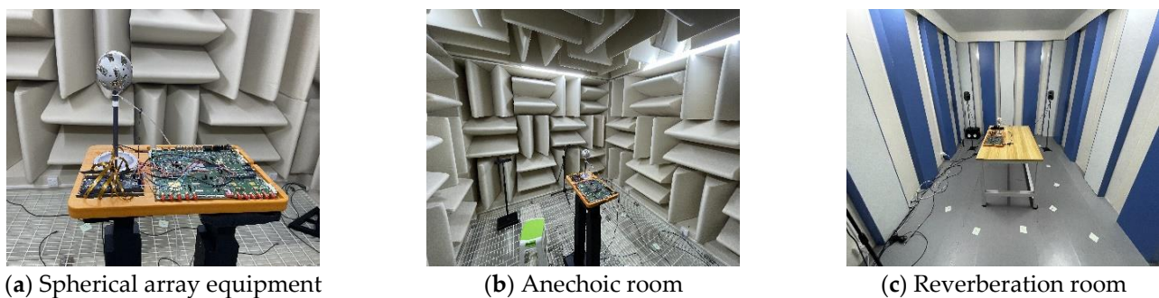
Figure 9. Experimental equipment and different field-testing scenarios.
