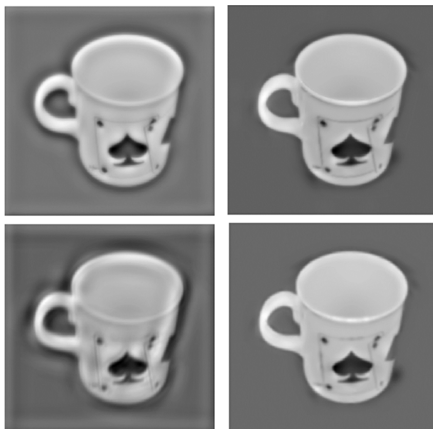
Figure 5: Image coding based on wavelets (left) and the brightness model (right). In both cases a limited number of scales has been used (top), which leads to severe rippling in the case of coding. If from all information only half is randomly selected, the coding result further deteriorates (bottom-left) but not the brightness result (bottom-right)
