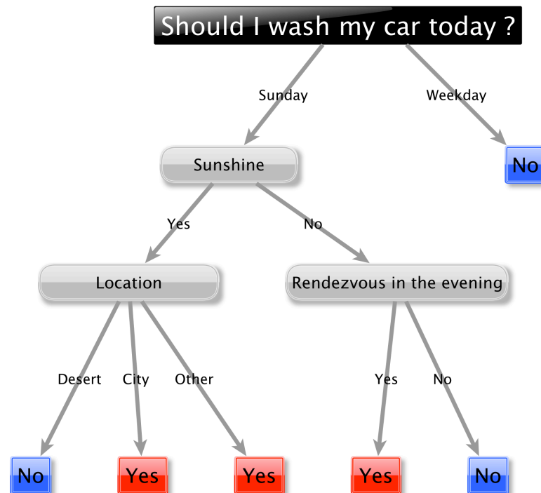
Figure 8. A decision tree for a binary decision problem. Although the decision problem is binary, the tree does not have to be binary too.
