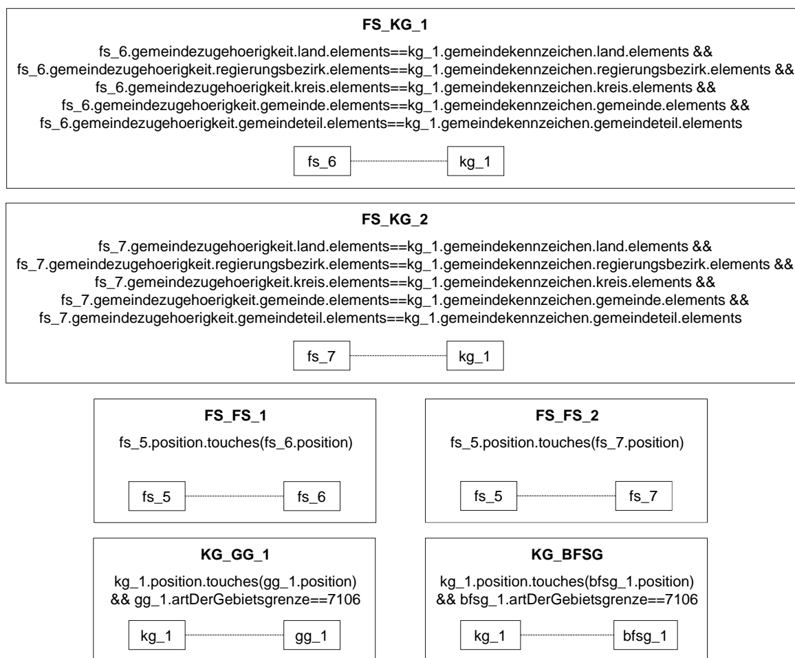
Figure D.2: VirtualAssociations from the UMLT transformation definition between AAA and INSPIRE
