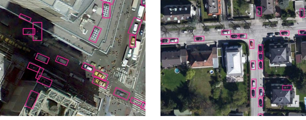
Figure 3. Output of the car detector. This task is challenging due to the small resolution of the target objects. The left image was captured from Google Earth while the right is part of the Bavaria dataset which was used for training the detector.
