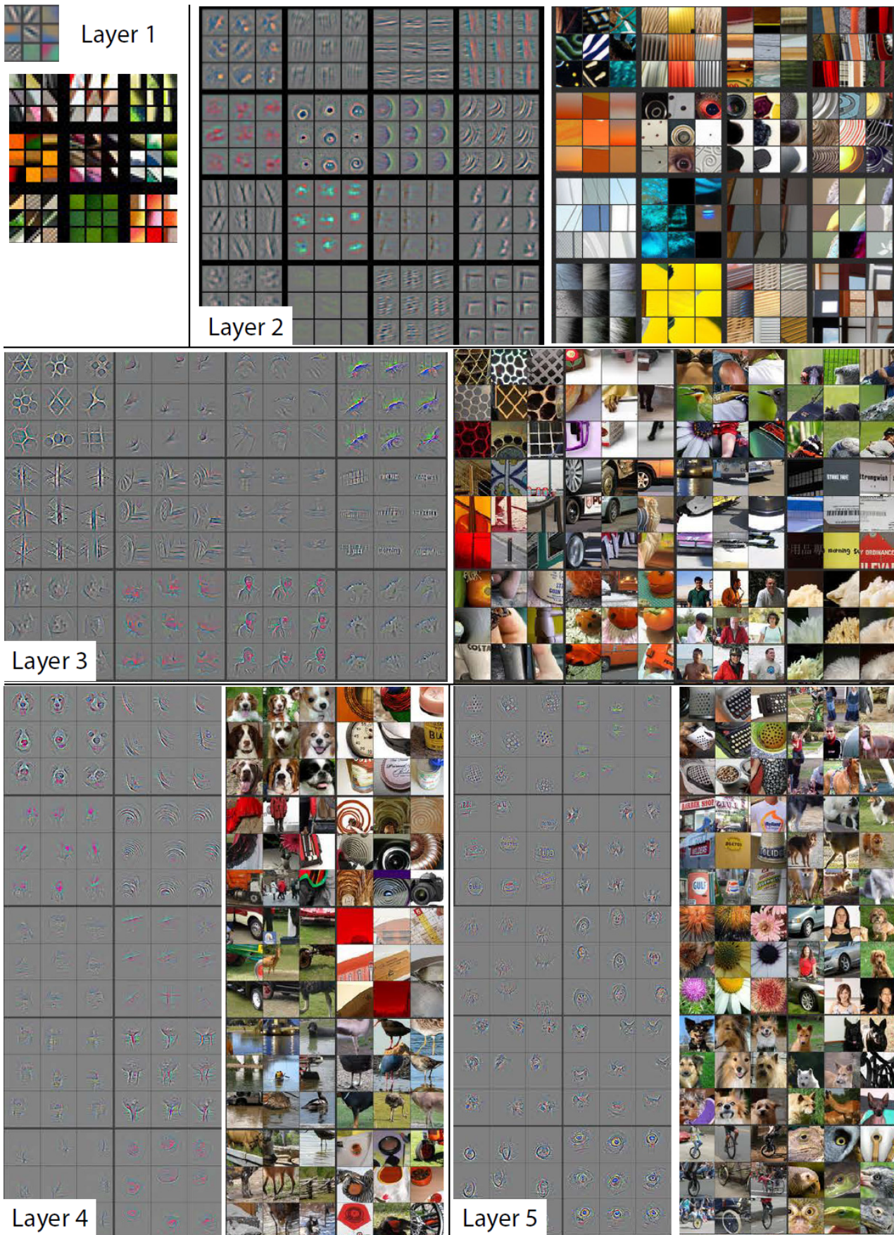
Fig. 9. From (Zeiler and Fergus, 2014). Visualizing different layers of a deep convolutional neural network. The left images show reconstructed patterns which cause high activations in a feature map. The right images show the corresponding image patches. The reconstructed patterns are projected down to pixel space using the deconvolutional network approach of (Zeiler and Fergus, 2014). The first layers extract simpler features (e.g. edges, corners, etc.), while the later layers describe complex shapes with greater variance.
