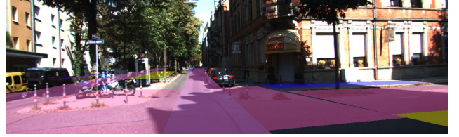
Fig. 40. Visualization of our semantic road parsing results using only aerial images. The road lanes are shown with shades of pink, the sidewalk with blue and the parking spots with yellow.
