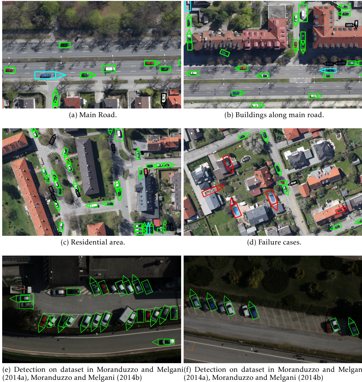
Fig. 21. Detection results from the DLR test images. Green and cyan bounding boxes are the correct detected samples, representing cars and trucks, respectively. Black bounding boxes are the missed ones and red are the false positives. The results show that our method works well in most scenarios (a)(b)(c), however the complicated rooftops or outdoor swimming pools may lead to false positive detections (d). We also evaluated our method on the dataset presented in Moranduzzo and Melgani (2014a), Moranduzzo and Melgani (2014b), the detection results are shown in (e)(f).
