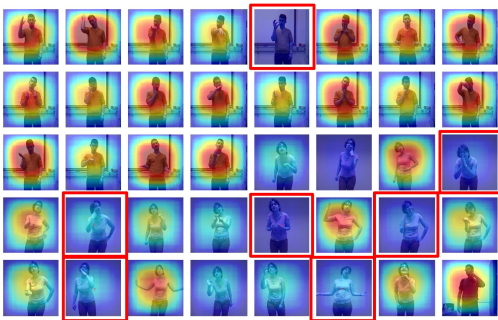
Figure 5.11: The 2D heat maps of the dominant positions of the first 40 gesture segments in the testing dataset. Each 2D heat map is corresponding to one gesture segment. The 2D heat maps are obtained by aggregating the spatial region of the spatio-temporal block of all the tree nodes in the random forest weighted by the probability of the corresponding gesture class. Red rectangles mean the mis-classified gesture segments. Red indicates high frequency and blue indicates low frequency (best viewed in color).
