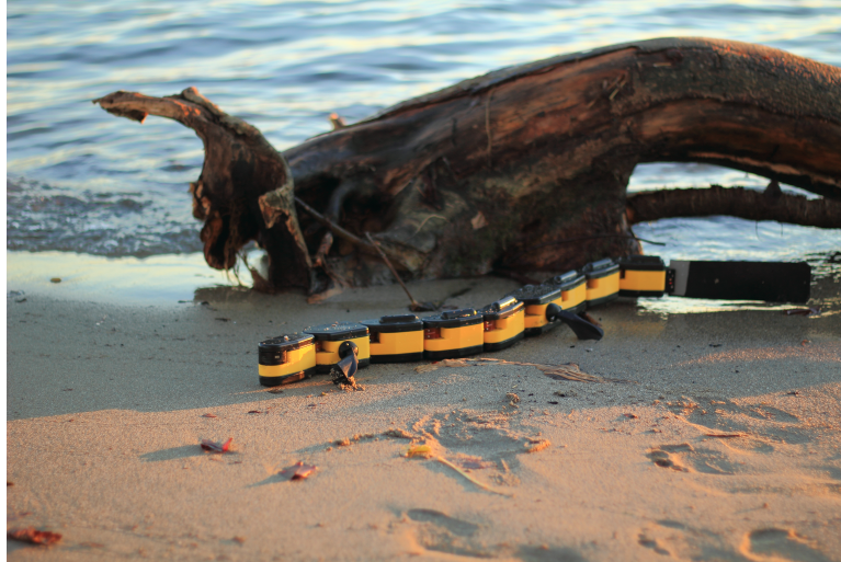
Figure 2.12: Salamander robot developed by Ijspeert [204].
