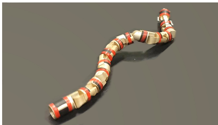
Figure 7.1: The snake-like robot is slithering forward. This snake-like robot is modular designed. Each joint axis is orthogonal to its neighbors with a rotation range of \pm 90^\circ .
