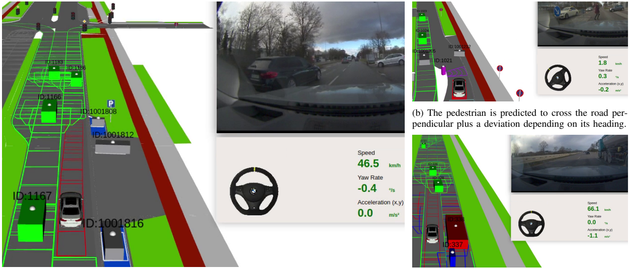
(a) Even on multi-lane roads, the ego vehicle has enough free space, since the safe distance forbids passing vehicles from merging directly in front of the ego vehicle. (b) The pedestrian is predicted to cross the road perpendicular plus a deviation depending on its heading. (c) While overtaking a truck, a vehicle ahead is merging into the lane of the ego vehicle.
