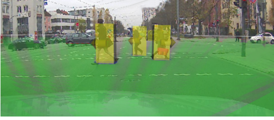
Fig. 5. View from the front camera of the autonomous vehicle approaching three pedestrians crossing the street. The recorded data is provided by [30].
