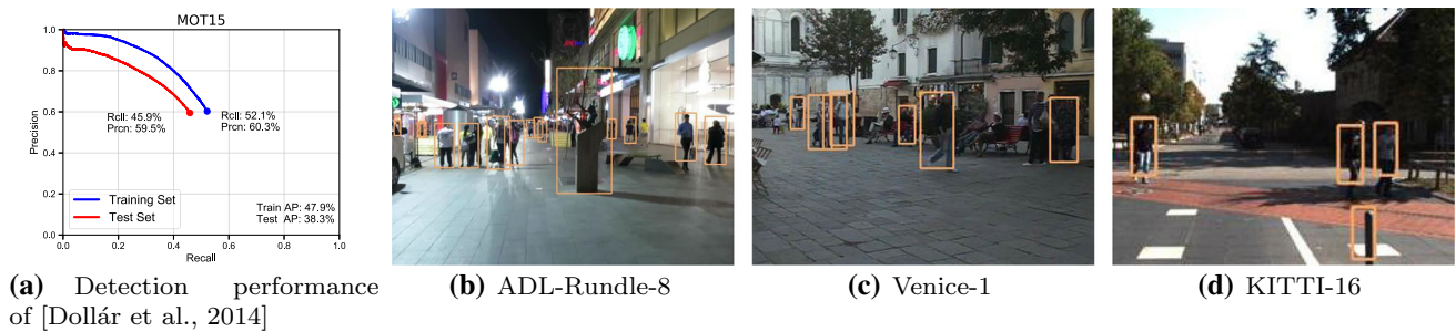
Fig. 2 a The performance of the provided detection bounding boxes evaluated on the training (blue) and the test (red) set. The circle indicates the operating point (i.e., the input detection set) for the trackers. b–d Exemplar detection results
