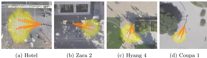
Fig. 5: Visualisation of generated trajectories (orange circles) and estimated global goal probabilities (yellow heatmap). The figures show that the model interacts with the visual context of the scene and ensures feasibility predictions.
