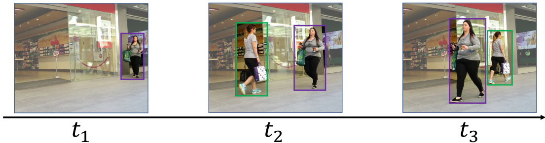
Figure 11: Visualization of a pedestrian tracking scenario. The multi-object tracking task involves detecting and localizing objects of interest and associating them across different timesteps.
