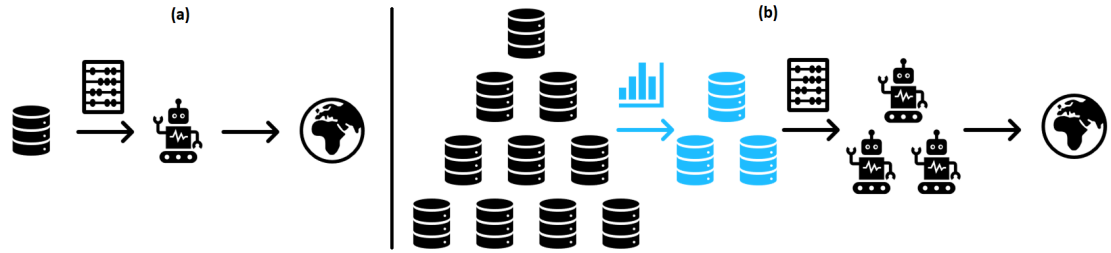
Figure 4.1: Schematic of the newly proposed dataset selection problem in offline RL: In Figure (a), the standard offline RL process is shown, where a single dataset is provided and an agent is distilled from it via some learning algorithm, before it is finally deployed in the real environment. In Figure (b) we are provided with many datasets from different systems, introducing the problem of how to select the most promising ones for offline RL. In a new step, a subset of the datasets is selected by calculating quality metrics for all of them. Finally, the selected datasets are again used to train policies which can be deployed.
