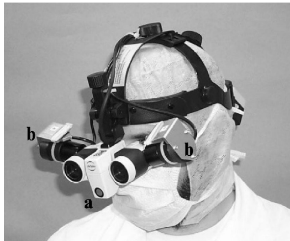
Figure 1.6: Augmented binoculars by Birkfellner et al. [19]. ©2002 IEEE.
