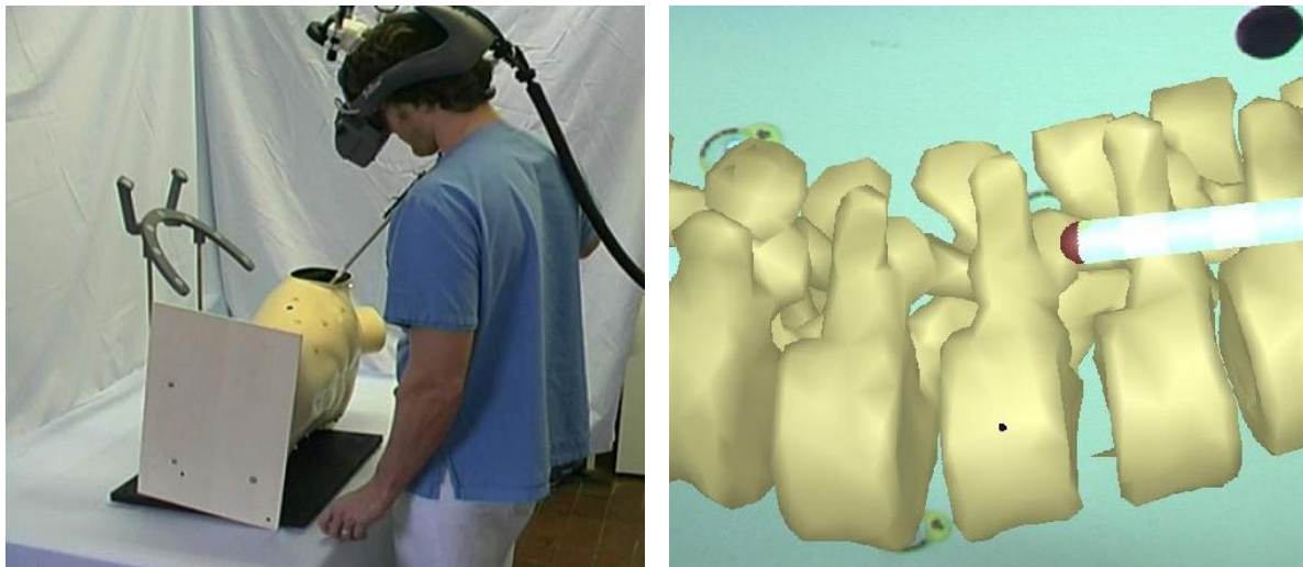
Figure 4.18: Augmented surgical instrument serves as the pointer device. The small black point is visualized. The surgeons were asked to touch the point with its tip in the virtual position.
