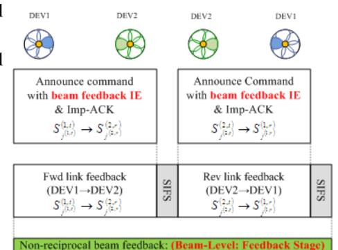
DEV1 ( $K^{(1,t)}$  transmit beams,  $K^{(1,r)}$  receive beams) and DEV2 ( $K^{(2,t)}$  transmit beams,  $K^{(2,r)}$  receive beams)
