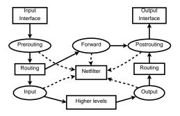
Fig. 4. The packet filter mechanism
