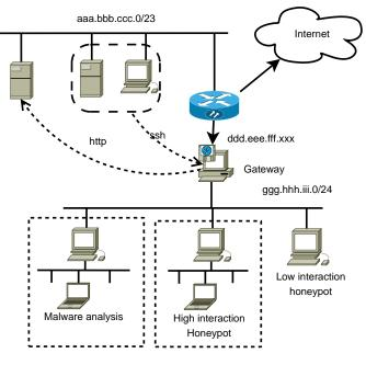
Fig. 1. Architecture of the platform
