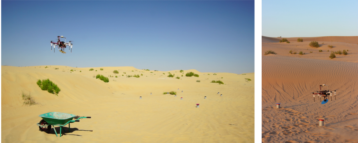
Figure 16: Photos from the tests of the proposed system in the desert near Abu Dhabi, United Arab Emirates. The grasping procedure is captured in the image on the right, and the dropping maneuver is shown in the image on the left. http://mrs.felk.cvut.cz/jfr2018treasurehunt-video3
