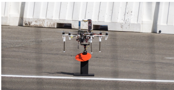
(c) Photo of a UAV grasping a static object from the stand.
