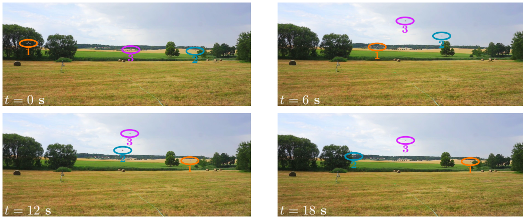
Figure 15: MPC-based collision avoidance between three drones. Two drones (UAV 1 and UAV 2) exchange their positions, while the third UAV 3 hovers in a position colliding with their trajectories. Using MPC future trajectory prediction, the UAVs avoid a collision by changing their trajectory height. http://mrs.felk.cvut.cz/jfr2018treasurehunt-video2
