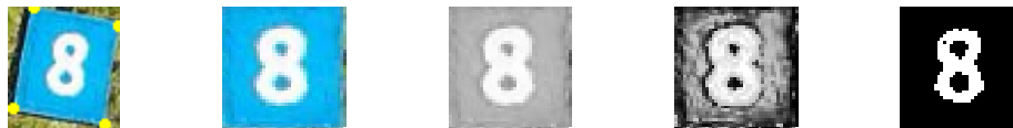
Figure 10: Digit recognition stages from left to right: image provided by the detection system with indicated corners, transformed image, grayscaled image, result of histogram equalisation, and thresholded image
