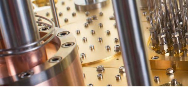
The Proteox<sup>™</sup> Secondary Insert is a customisable, self-supporting module to enable installation and exchange of full experimental set-ups.
