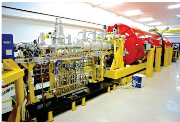
Figure 1 : The fully refurbished EN tandem accelerator.
