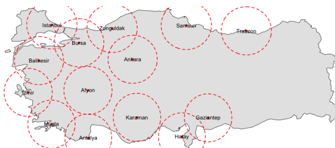
Figure 2. The distribution of 14 radar network over Turkey. Precipitation products of six radars (Istanbul, Bursa, Balıkesir, İzmir, Muğla, and Afyon), which were taken from TSMS were evaluated manually to describe the characteristics of the precipitation types.
