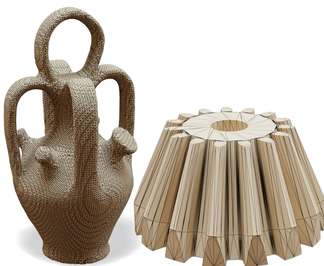
Figure 2.1: An intrinsic triangulation exactly preserves the input geometry, while changing the mesh connectivity. Hence, if the input mesh gives an exact description of the geometry (as with the CAD model at right), it will not be corrupted; if the input exhibits noise or approximation error (as with the marching cubes approximation at left), these errors will get neither better nor worse.
