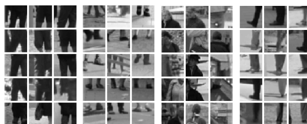
Figure 1. Large-scale features learned by the proposed model for pedestrian detection. Each plate corresponds to a set of image patches with highest compatibility with a feature.
