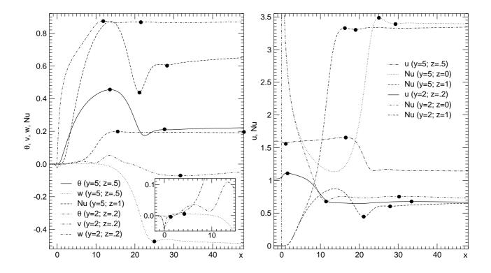
Figure 3: Longitudinal profiles of  $\theta$ , u, v and w along the lines at (y, z) = (2, 0.2) and (5, 0.5) and longitudinal profiles of  $Nu_t$  and  $Nu_b$  along the lines at y = 2 and y = 5. These profiles are the same for the four contributors. The filled circles indicates the local extrema whose values and coordinates are given in Tables 3 and 4.
