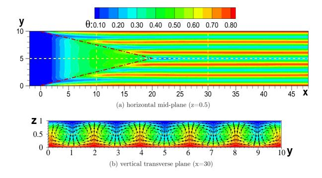
Figure 2: Temperature fields,  $\theta$ , in the horizontal mid-plane and temperature field and velocity vector field in the transverse plane at x=30 in the longitudinal roll flow of the present test case. The yellow dashed lines are some of the lines along which  $\theta$ , u, v and w profiles and their extrema are calculated. The red dash-dotted lines border the forced convection triangular zone at the entrance of the heated plate, in which no thermoconvective rolls are present.
