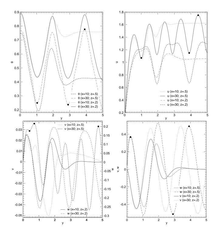
Figure 4: Spanwise profiles of the primitive variables  $\theta$ , u, v and w obtained by the four contributors along the lines at (x, z) = (10, 0.2), (10, 0.5), (30, 0.2) and (30, 0.5). The filled circles indicates the local extrema whose values and coordinates are given in Table 3.
