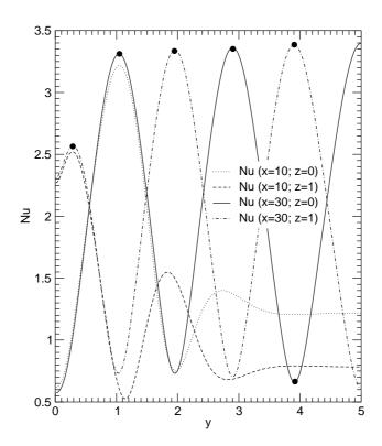
Figure 5: Transverse profiles of the Nusselt numbers  $Nu_t$  and  $Nu_b$  obtained by the four contributors along the lines at x = 10 and x = 30. The filled circles indicates the local extrema whose values and coordinates are given in Table 4.
