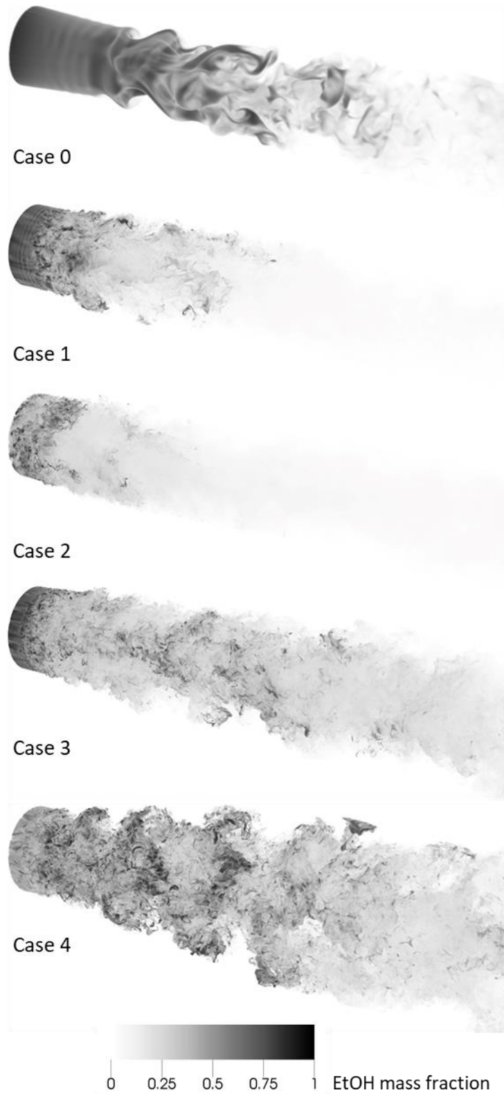
Fig 4. Instantaneous concentration volume renderings for the cases 0 to 4 (top to bottom) - see additional videos 2-6. The turbulent transitions of the coaxial jets is due to the significant development of primary and secondary Kelvin Helmholtz instabilities resulting from strong shear stress between layers of different densities. DNS emphasizes the multitude of scales and highlights the
