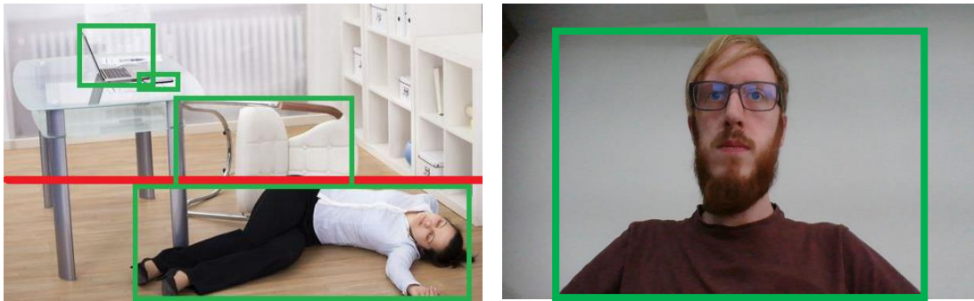
Figure 4.3. The left image shows where the floor threshold is set on this image. Identifying a person below this triggers the fall detection framework. The objects on the desk are not below this threshold, therefore will not be triggered or identified as a hazard.
