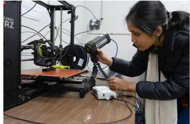
Image 1. Rifat-E-Nur Hossain, a Ph. D. student at Louisiana Tech University and Louisiana Materials Design Alliance (LAMDA) research, prepares a thermal camera for image capture during operation of a 3D printer. Source: Louisiana Tech University.
