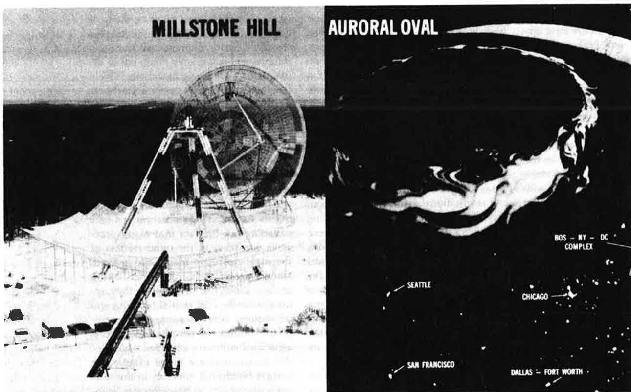
Studying the upper atmosphere. The new 46-meter fully steerable radar antenna at Millstone Hill, Massachusetts, is seen behind the older, fixed, vertically pointing 67-meter antenna. The instruments are used for studying the sources and dynamics of magnetospheric phenomena, the best known of which is the spectacular aurora circling the polar regions, shown in this satellite picture.
