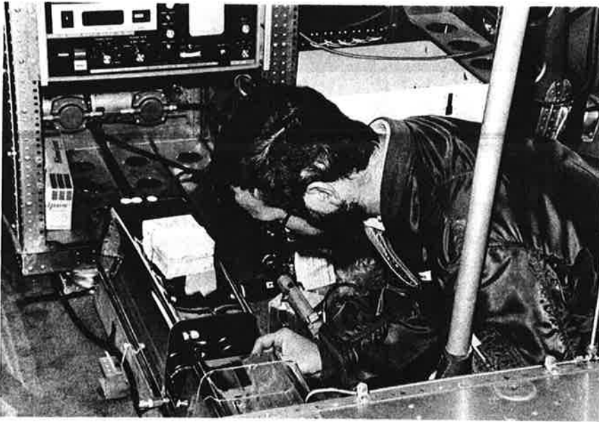
Monsoon studies. Anthony Delany calibrates a spectrometer aboard NCAR's Electra aircraft as part of the winter phase of the 1979 MONEX. The laser instrument identifies the sizes and types of particles suspended in the air, information used in trying to understand the relationship of monsoons to global weather.
