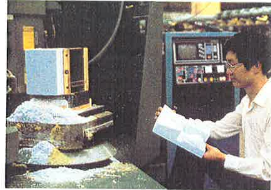
Engineering Research Centers. Ohio State University work involves the computer-aided design and machining of polystyrene models for making dies. Completed model is shown in photo immediately below. At Lehigh University, the Center for Advanced Technology for Large Structural Systems is examining such structures as New York City's Javits Convention Center, shown in second photo.
