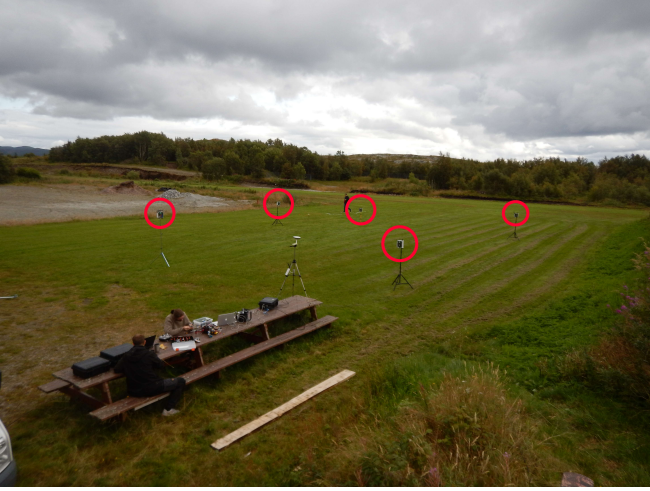
Fig. 4: UWB Anchor constellation view during field flight tests
