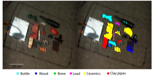
Fig. 7 UHI images of metal frame with OOI deposited on the seabed adjacent to the reference wreck. Image to the right shows SAM classifications based on spectral library created in laboratory (misclassifications of the white reference plate and nylon rope have been removed).
