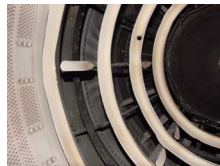
Ceramic Coated Liner and Flame Holders Implementation of MSZ TBC Allowed Continuous Use of Afterburner and First Sustained Flight Above Mach III of an Air Breathing Engine
