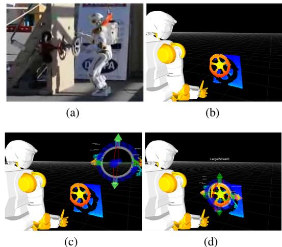
Figure 1: Placing a wheel-turning template in RViz.
