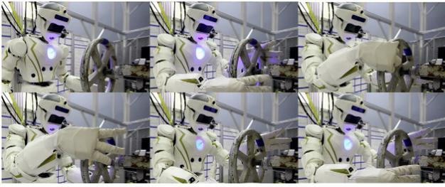
Figure 2: Turning a valve using an affordance template.
